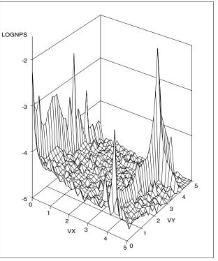
Figure 5. Two-dimensional NPS of Digital Printer Flat Field.
