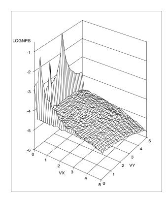
Figure 2. Two-dimensional NPS of Synthetic Pattern. The frequency axes are [0-5 cy/mm].
