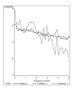
Figure 6. Streaking and Granularity NPS for Digital Printer Flat Field
